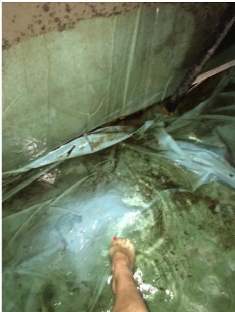
Bubbles in the bladder feel like they are full of air, but it is water pushing the bladder up from the floor of the tank.
